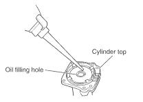
Apply grease to the inside of the cylinder cup and to the O-ring and shaft of the air piston, and then reassemble by following the disassembly procedure in reverse.
