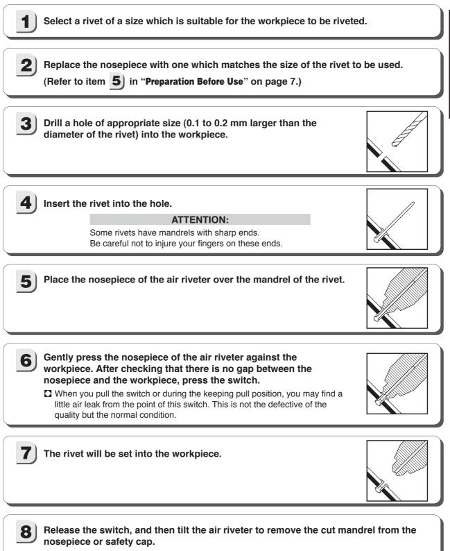
NOTE: Make sure that the cut mandrel has been completely removed before proceeding to the next riveting.
