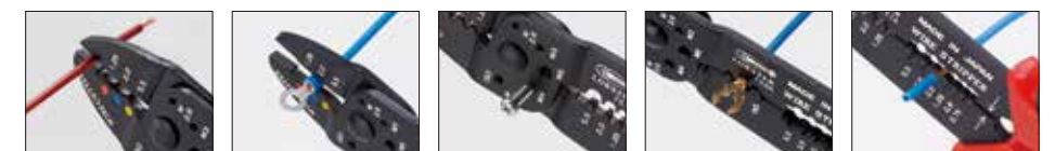
Wire cutter Crimp tooth opening for insulated terminal (Insertion terminal: 1.25mm, 2mm) Bolt cutter (Applicable size: M2.6 to M5) Crimp tooth opening for open barrel terminal (Insertion terminal: 1.25mm, 2mm) Wire stripper (Applicable size: 0.75 to 5.5mm)
