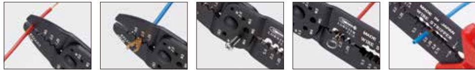
Wire cutter Crimp tooth opening for open barrel terminal (Insertion terminal: 1.25mm, 2mm) Bolt cutter (Applicable size: M2.6 to M5) Crimp tooth opening for non-insulated crimp terminal and P.B sleeve (1.25mm, 2mm, 5.5mm) Wire stripper (Applicable size: 0.75 to 5.5mm)
