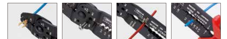
Crimp tooth opening for open barrel terminal (Insertion terminal: 1.25mm, 2mm) Bolt cutter (Applicable size: M2.6 to M5) Wire cutter Wire stripper (Applicable size: 0.75 to 5.5mm)
