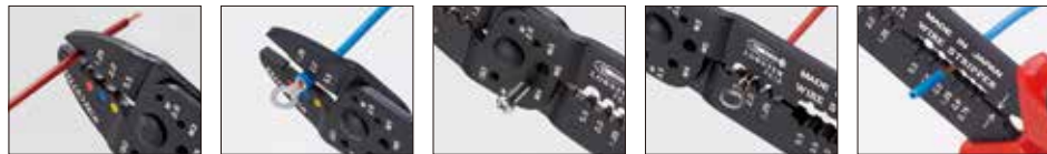
Wire cutter Crimp tooth opening for insulated terminal (Insertion terminal: 1.25mm, 2mm) Bolt cutter (Applicable size: M2.6 to M5) Crimp tooth opening for non-insulated crimp terminal and P.B sleeve (1.25mm, 2mm, 5.5mm) Wire stripper (Applicable size: 0.75 to 5.5mm)
