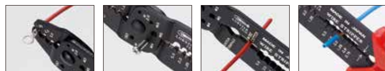
Crimp tooth opening for non-insulated crimp terminal and P.B sleeve (1.25mm, 2mm, 5.5mm) Bolt cutter (Applicable size: M2.6 to M5) Wire cutter Wire stripper (Applicable size: 0.75 to 5.5mm)
