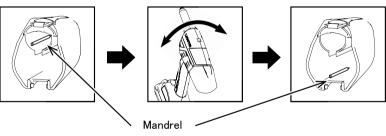
The cut mandrel may protrude from the nose piece tip, but this is not a malfunction.
