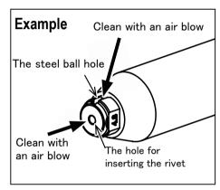
After cleaning, apply a low-viscosity lubricant to the steel ball hole and reassemble. Wipe off the overflowing lubricating oil.
