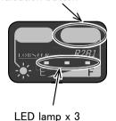
LED lamp lighting condition Contents of indication Left Center Right Remaining battery power of Lit Lit Lit 100 to 70% Remaining battery power of Lit Lit 70 to 30% Remaining battery power of Lit below 30% No battery power remaining \*1 Blinking Battery pack unattached \*2 Blinking Blinking Safety device activation \*1
